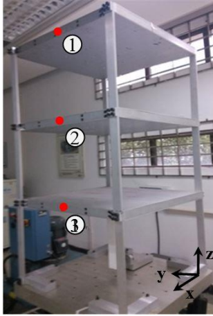
Fig. 4 The 3-story structure model and layout of sensors
