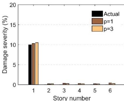
Fig. 9 Damage detection results for the tested structure in the damaged state (damage pattern I)
