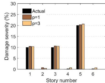
Fig. 11 Damage detection results for the tested structure in the damaged state (damage pattern III)
