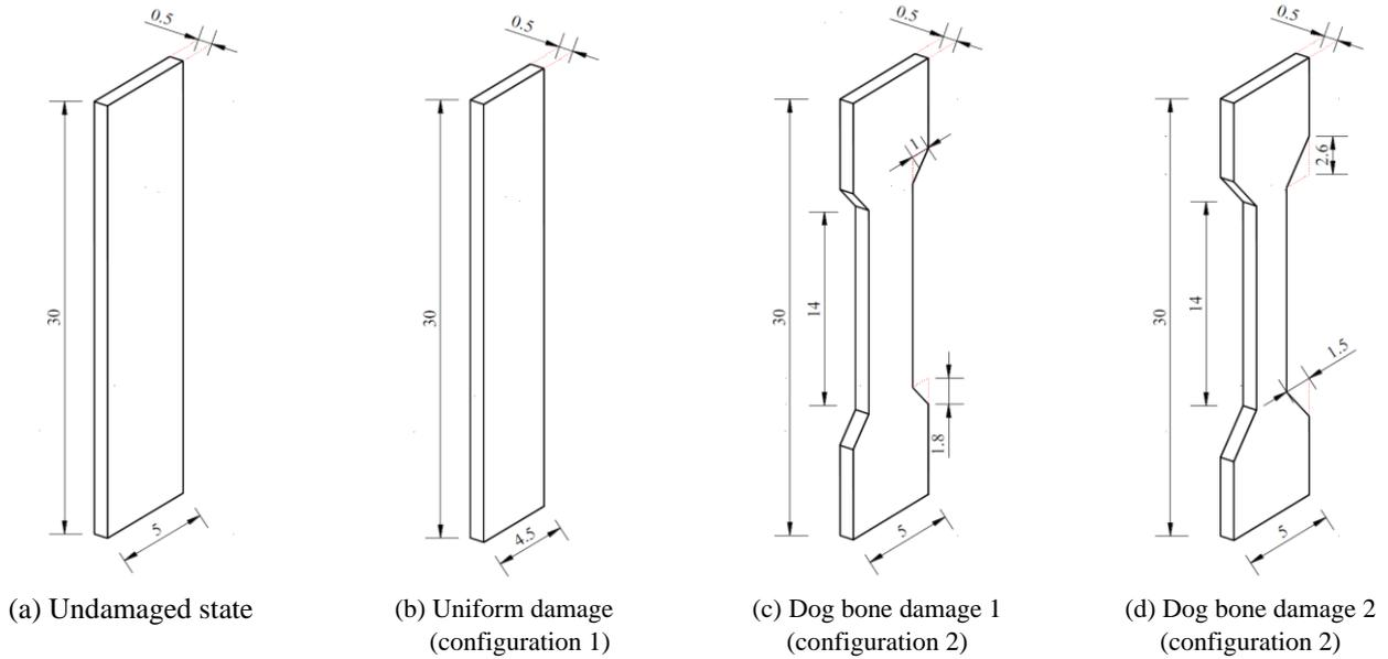
Fig. 7 Details of the column shapes used in the experimental study
