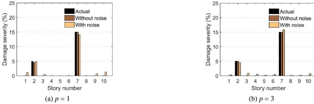
Fig. 2 Damage detection results for the second damage pattern of the numerical study
