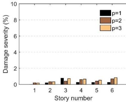
Fig. 8 Damage detection results for the tested structure in the intact state
