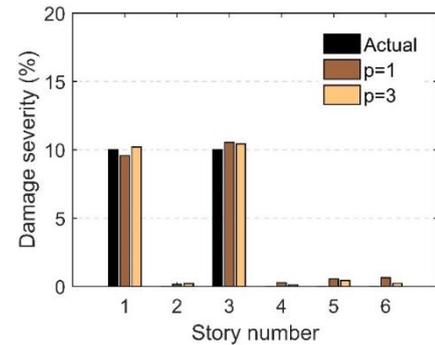
Fig. 10 Damage detection results for the tested structure in the damaged state (damage pattern II)
