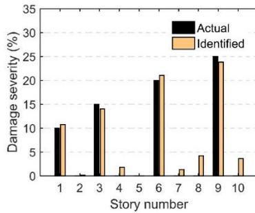
(a) Damage detection results using PSO
