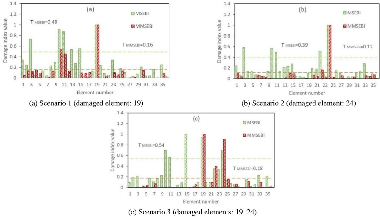
Fig. 20 The normalized MSEBI and MMSEBI comparison for the 36- bar spatial truss for sensor pattern 1 considering 7 modes with 7% noise
