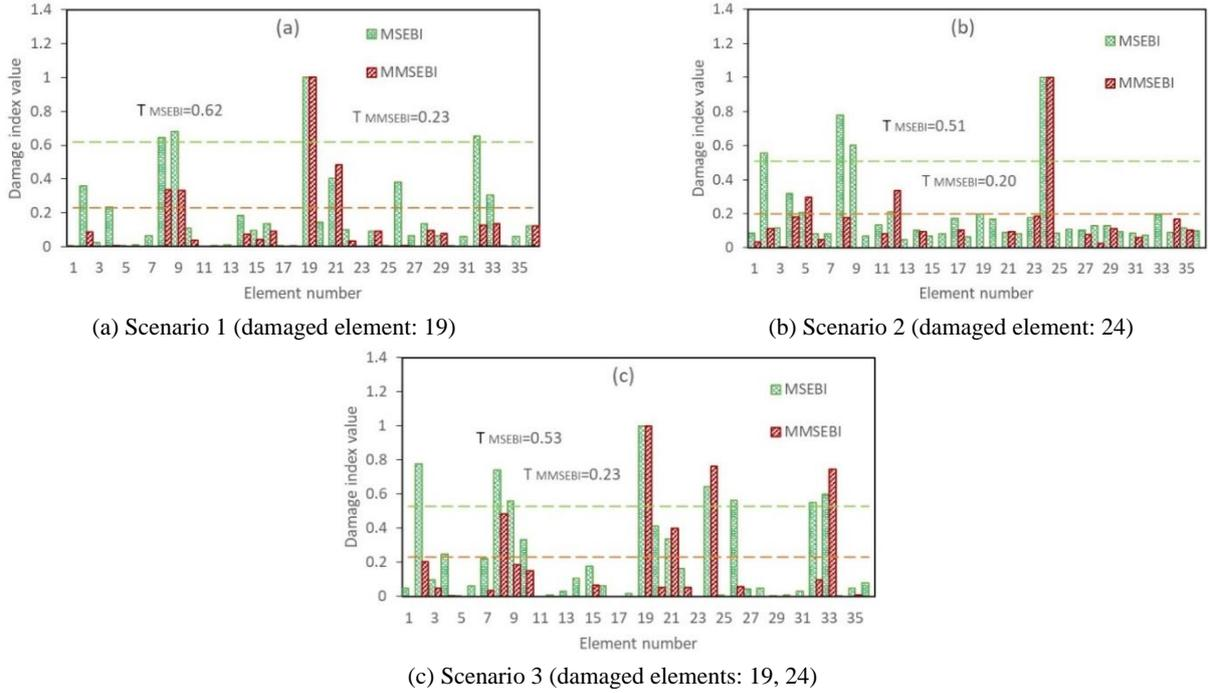
Fig. 23 The normalized MSEBI and MMSEBI comparison for the 36-bar spatial truss for sensor pattern 2 considering 5 modes with 3% noise
