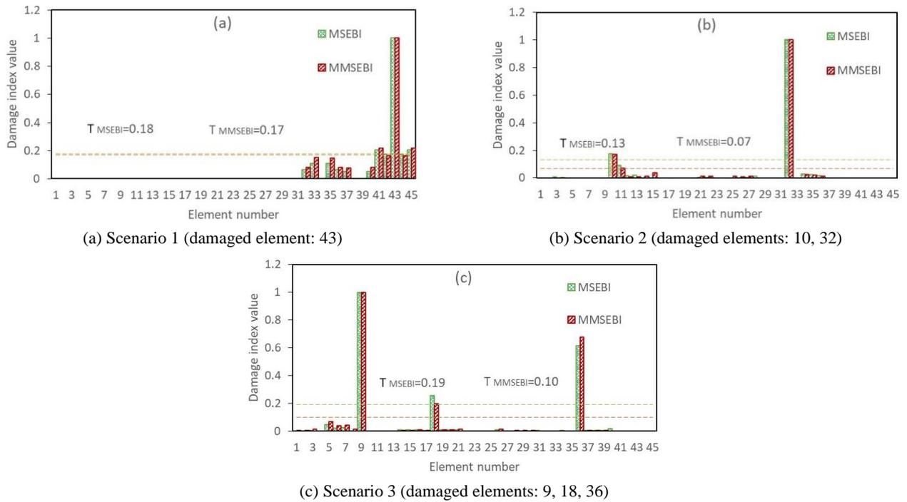
Fig. 8 The normalized MSEBI and MMSEBI comparison for the 45-element planar frame for sensor pattern 2 considering 3 modes without noise
