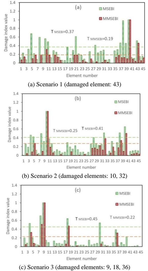
Fig. 4 The normalized MSEBI and MMSEBI comparison for the 45-element planar frame for sensor pattern 1 considering 5 modes with 3% noise
