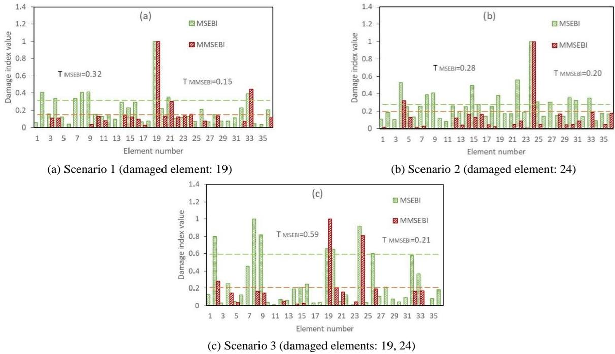
Fig. 26 The normalized MSEBI and MMSEBI comparison for the 36-bar spatial truss for sensor pattern 2 considering 7 modes with 7% noise
