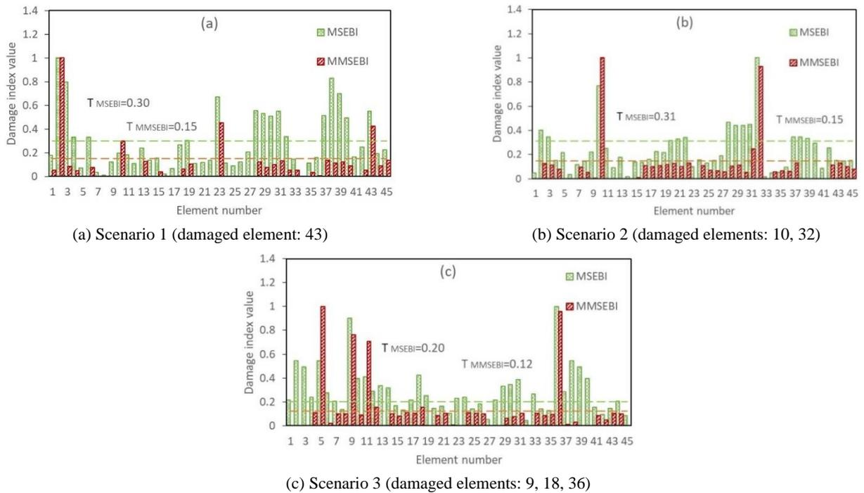
Fig. 12 The normalized MSEBI and MMSEBI comparison for the 45-element planar frame for sensor pattern 2 considering 5 modes with 7% noise
