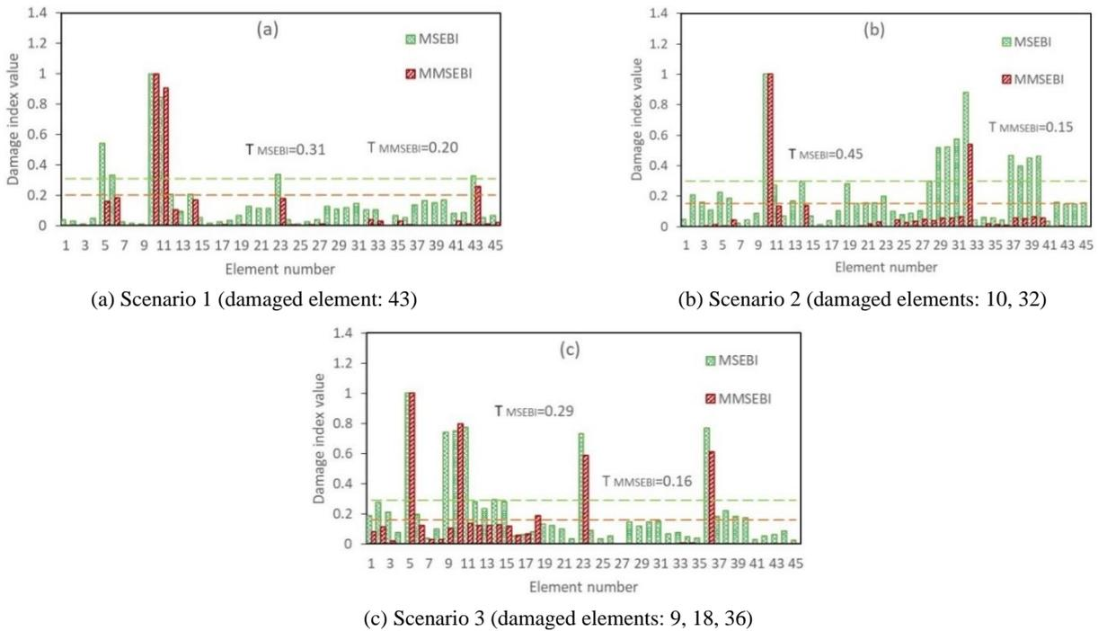
Fig. 10 The normalized MSEBI and MMSEBI comparison for the 45-element planar frame for sensor pattern 2 considering 5 modes with 3% noise
