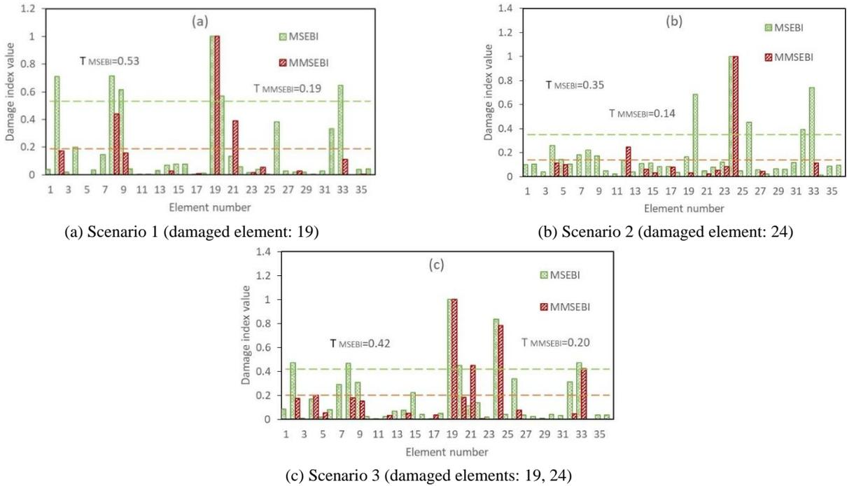
Fig. 24 The normalized MSEBI and MMSEBI comparison for the 36-bar spatial truss for sensor pattern 2 considering 7 modes with 3% noise
