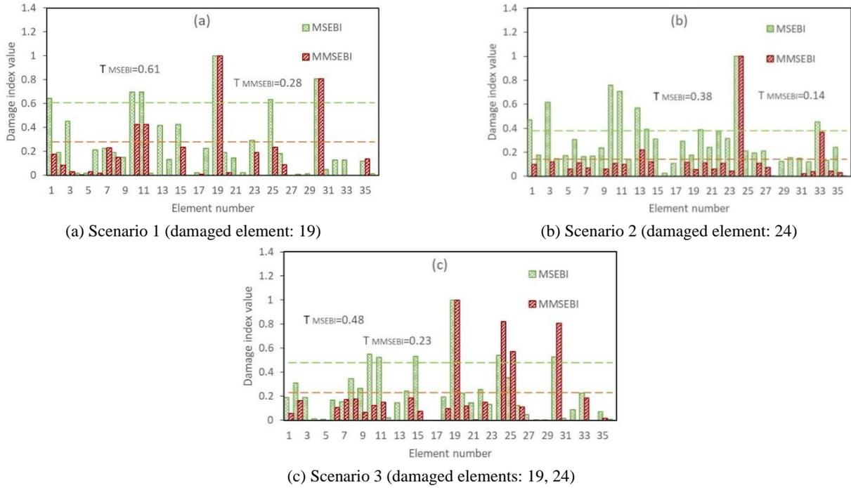
Fig. 19 The normalized MSEBI and MMSEBI comparison for the 36- bar spatial truss for sensor pattern 1 considering 5 modes with 7% noise
