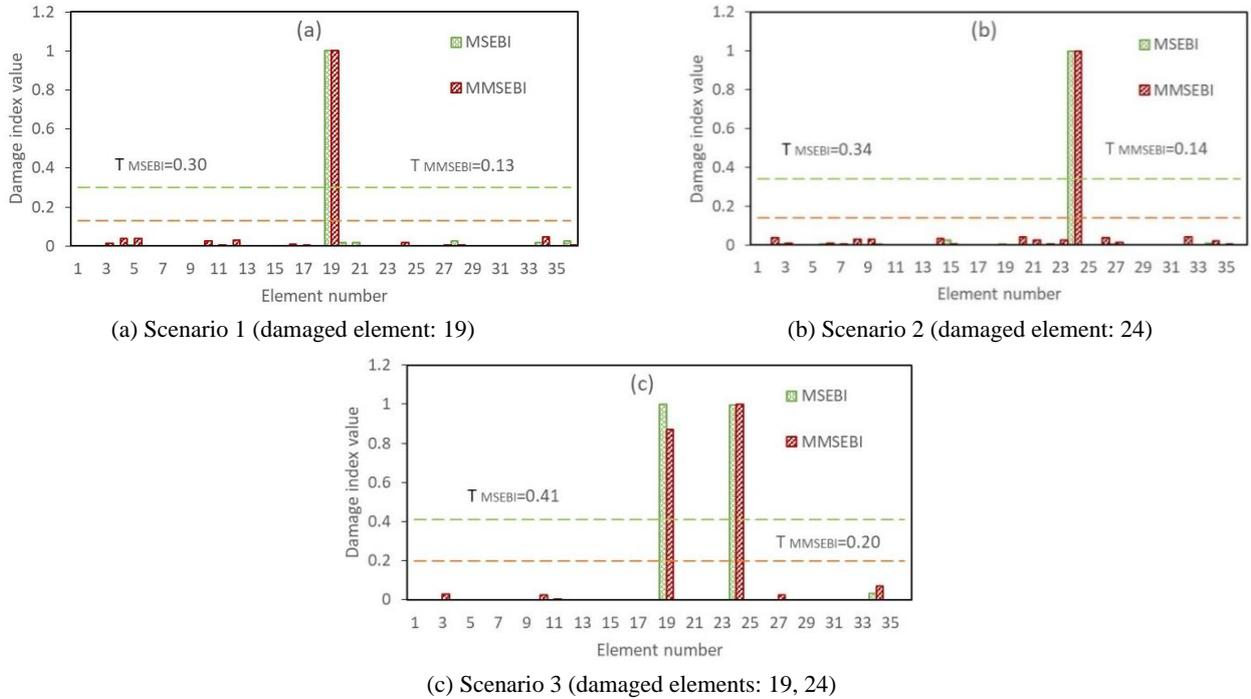
Fig. 16 The normalized MSEBI and MMSEBI comparison for the 36-bar spatial truss for sensor pattern 1 considering 4 modes without noise
