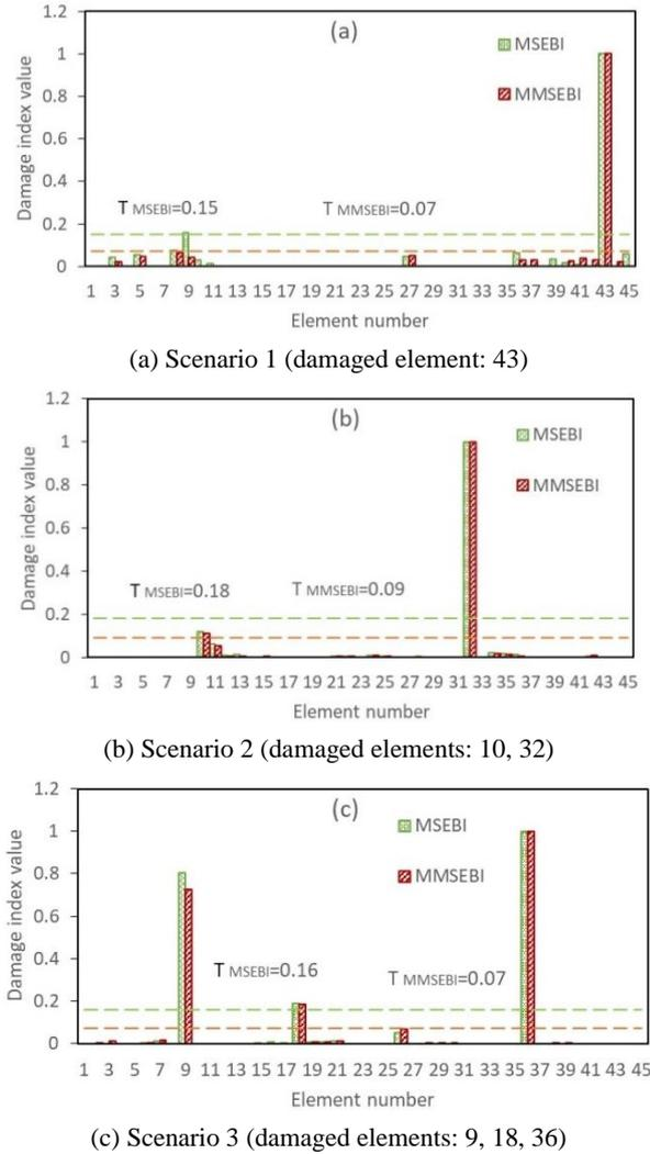
Fig. 3 The normalized MSEBI and MMSEBI comparison for the 45-element planar frame for sensor pattern 1 considering 5 modes without noise
