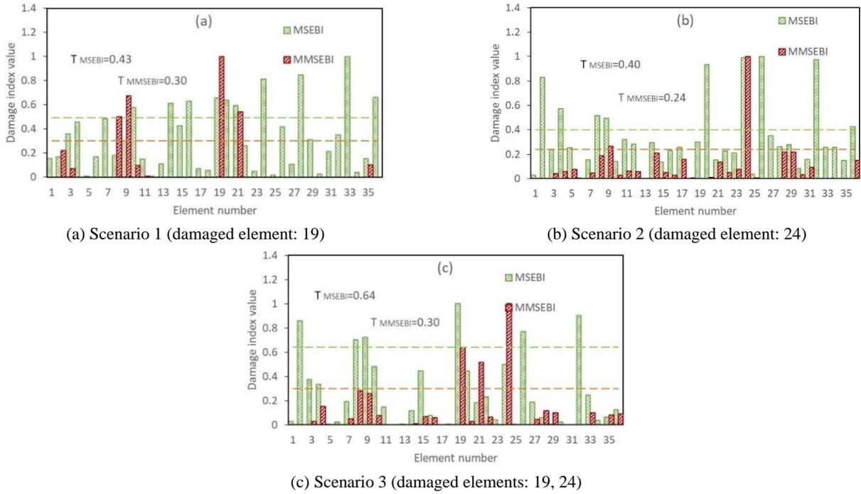
Fig. 25 The normalized MSEBI and MMSEBI comparison for the 36-bar spatial truss for sensor pattern 2 considering 5 modes with 7% noise
