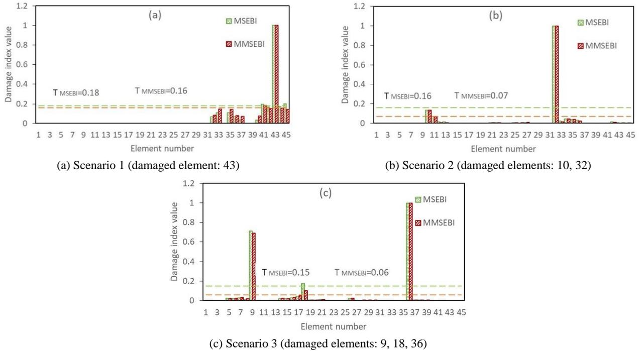
Fig. 9 The normalized MSEBI and MMSEBI comparison for the 45-element planar frame for sensor pattern 2 considering 5 modes without noise
