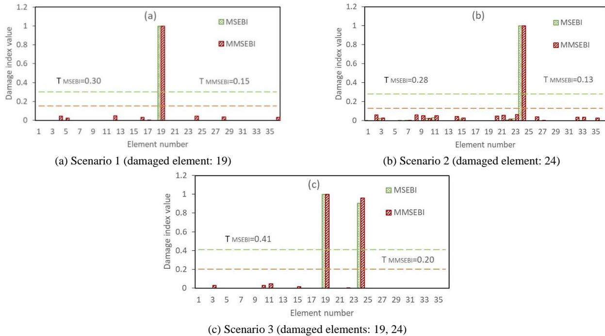
Fig. 22 The normalized MSEBI and MMSEBI comparison for the 36-bar spatial truss for sensor pattern 2 considering 4 modes without noise
