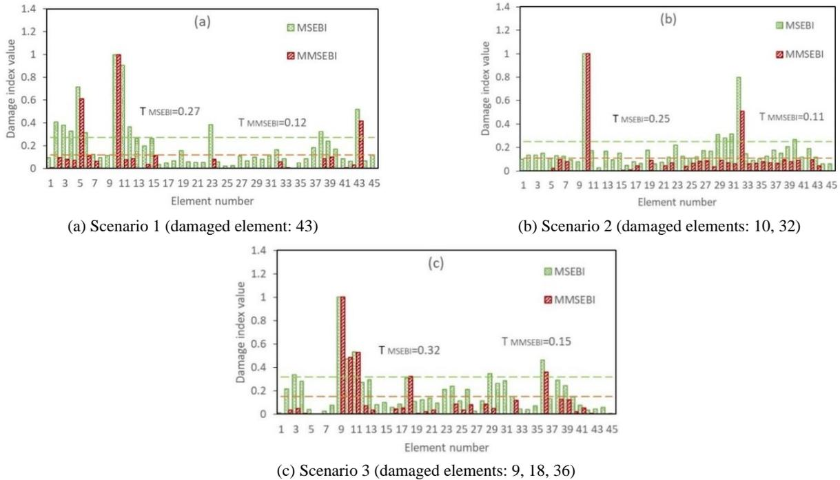
Fig. 13 The normalized MSEBI and MMSEBI comparison for the 45-element planar frame for sensor pattern 2 considering 7 modes with 7% noise
