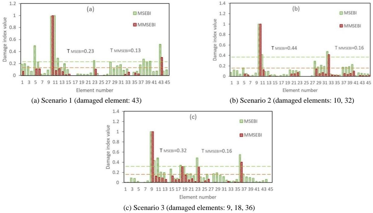
Fig. 11 The normalized MSEBI and MMSEBI comparison for the 45-element planar frame for sensor pattern 2 considering 7 modes with 3% noise
