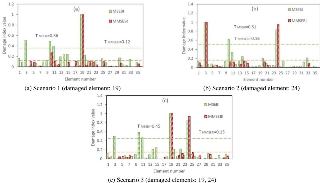
Fig. 18 The normalized MSEBI and MMSEBI comparison for the 36- bar spatial truss for sensor pattern 1 considering 7 modes with 3% noise
