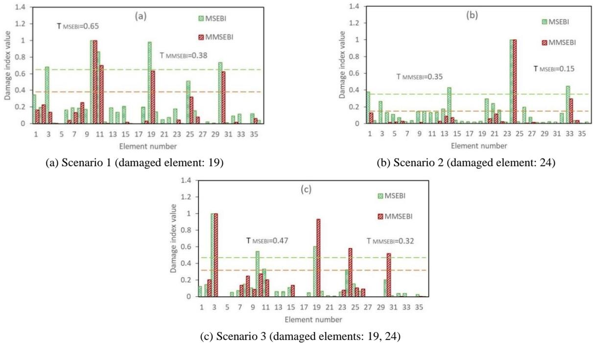
Fig. 17 The normalized MSEBI and MMSEBI comparison for the 36-bar spatial truss for sensor pattern 1 considering 5 modes with 3% noise
