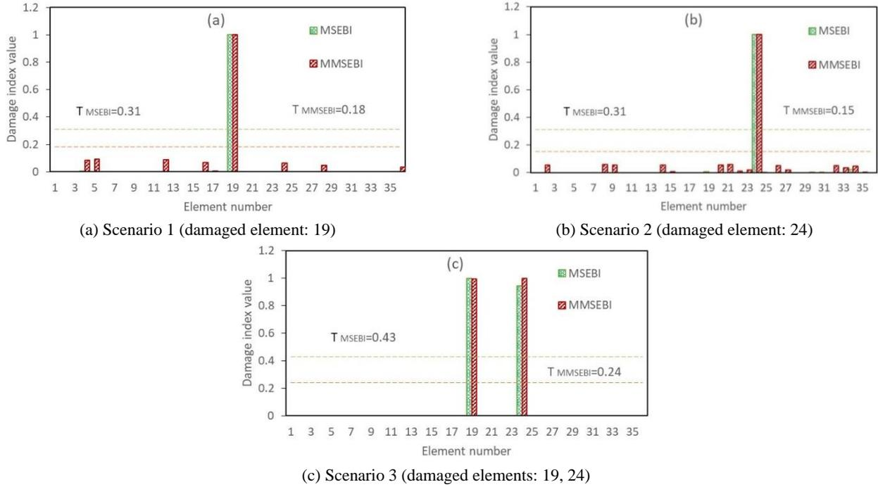
Fig. 21 The normalized MSEBI and MMSEBI comparison for the 36-bar spatial truss for sensor pattern 2 considering 3 modes without noise
