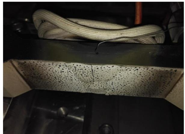
(b) The paint buckled in the final stages of the experiment
