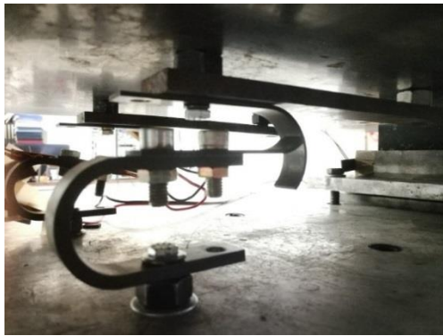
Fig. 13 Detail of the rupture of the thin U-shaped element
