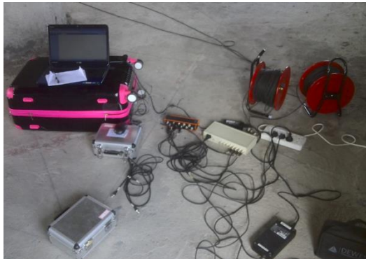
Fig. 5 Data acquisition system
