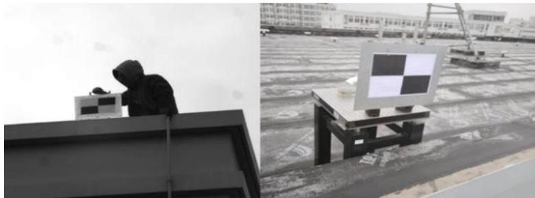
Fig. 6 Marker attached to a precision translation stage
