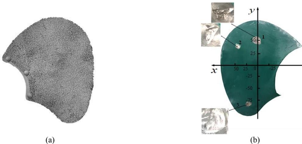
Fig. 4 (a) Speckle pattern and (b) three artificial damage on the fan blade
