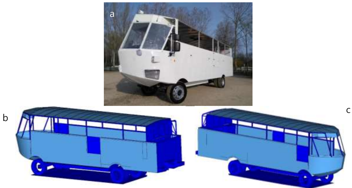
Fig. 1 (a) Prototype amphibious bus, (b) and (c) CAD and the finite element of the vehicle from the front and rear view
