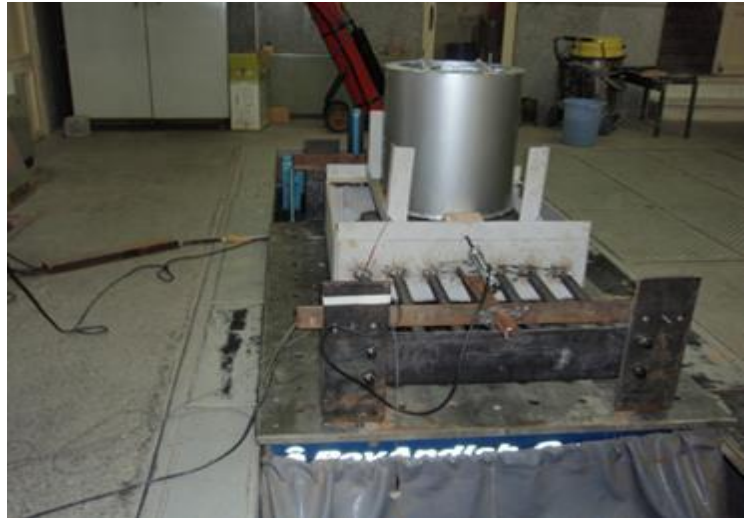
Fig. 2 Cylindrical TLD used for the SDOF structure connected to the shaking table
