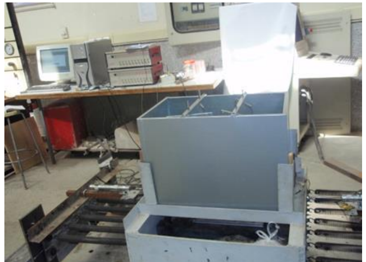
Fig. 3 Rectangular TLD used for the SDOF structure connected to the shaking table
