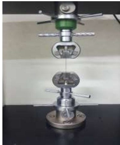
Fig. 3 Typical tensile test setup for the hysteretic tensile stress-strain behavior of SMA wires
