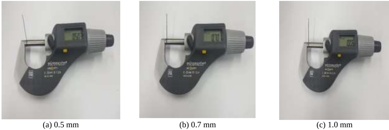
Fig. 2 Photographs of SMA fiber diameter measuring instruments
