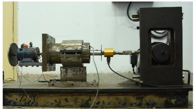
Fig. 3 Mechanical performance test setup of the REIMD
