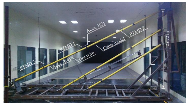
Fig. 1 The experimental setup of stay cable model
