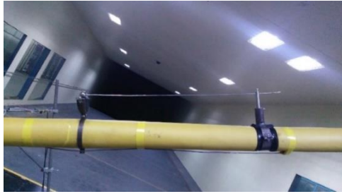
(b) PTMD-1 installed at the mid-span of the cable model
