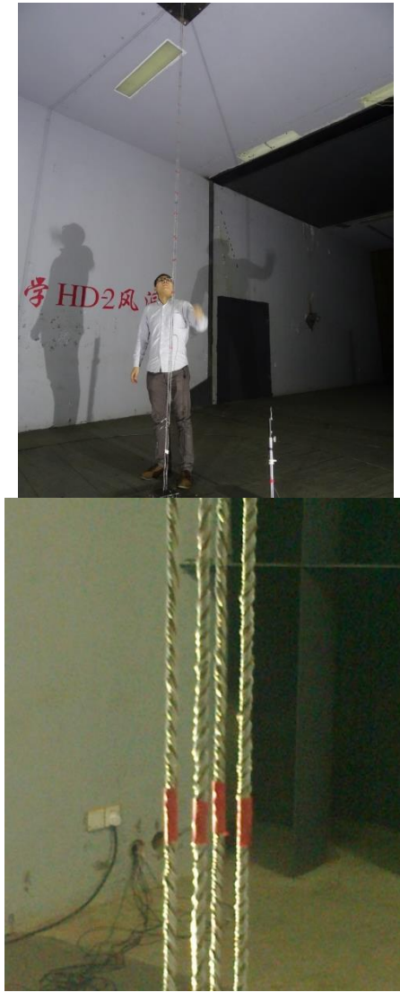
Fig. 7 Full aeroelastic model of parallel hangers in wind tunnel
