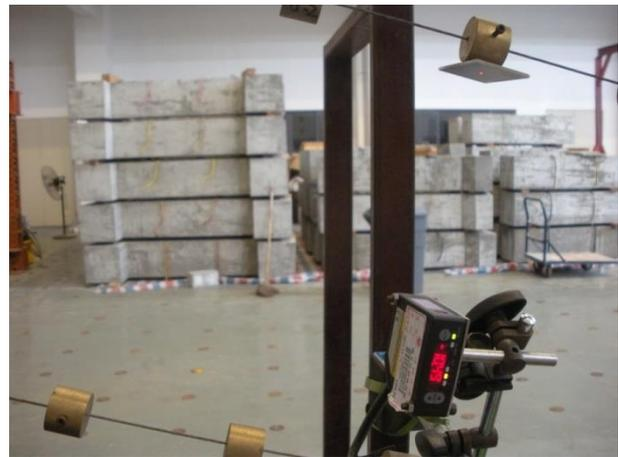
(b) Laser displacement sensor
