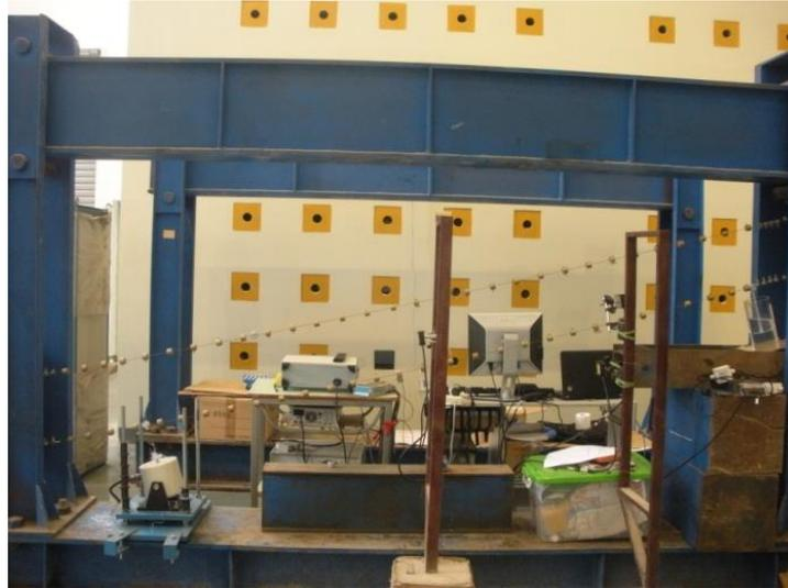
Fig. 6 Experimental setup of small-scale twin-cable system with a viscous damper
