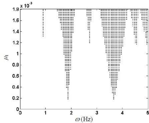
Fig. 6 Unstable region on the plane  $(\omega, \mu_1)$  of the controlled cable with multiple modes under random and periodic disturbances ( $\mu_2=0.05 \times 10^{-3}$ ,  $\zeta_{eq}=0.01$ )
