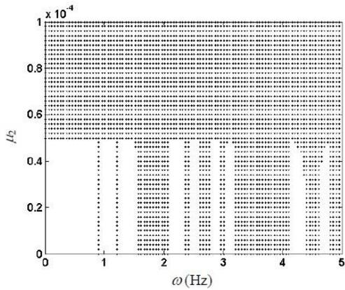
Fig. 15 Unstable region on the plane  $(\omega, \mu_2)$  of the controlled cable with multiple modes under random and periodic disturbances ( $\mu_1=1.5 \times 10^{-3}$ ,  $k_{eq}=0.2k_1$ )
