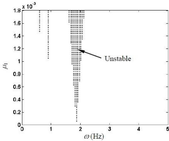
Fig. 2 Unstable region on the plane  $(\omega, \mu_1)$  of the uncontrolled cable with single mode under random and periodic disturbances ( $\mu_2=0.05 \times 10^{-3}$ )
