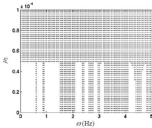
Fig. 14 Unstable region on the plane  $(\omega, \mu_2)$  of the controlled cable with multiple modes under random and periodic disturbances ( $\mu_1=1.5 \times 10^{-3}$ ,  $k_{eq}=0.1k_1$ )
