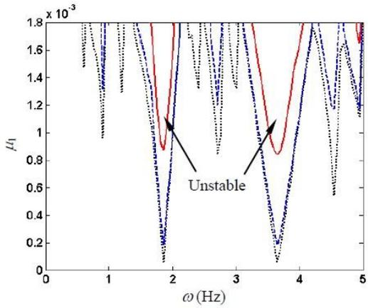
Fig. 8 Unstable region on the plane  $(\omega, \mu_1)$  of the controlled cable compared with the uncontrolled cable ( $\mu_2=0.05 \times 10^{-3}$ ) (solid line:  $\zeta_{eq}=0.05$ ; dashed line:  $\zeta_{eq}=0.01$ ; dotted line:  $\zeta=0.002$ )
