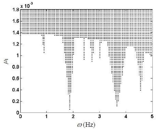
Fig. 11 Unstable region on the plane  $(\omega, \mu_1)$  of the controlled cable with multiple modes under random and periodic disturbances ( $\mu_2=0.05 \times 10^{-3}$ ,  $k_{eq}=0.1k_1$ )
