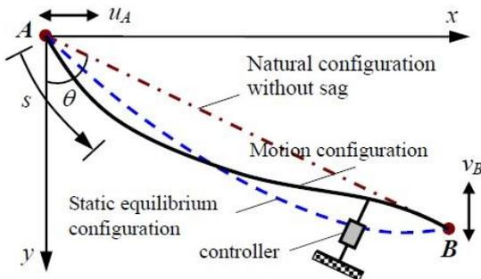
Fig. 1 An inclined sagged stay cable with control under support disturbances in plane
