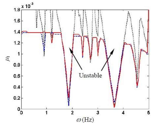
Fig. 13 Unstable region on the plane  $(\omega, \mu_1)$  of the controlled cable compared with the uncontrolled cable ( $\mu_2=0.05 \times 10^{-3}$ ) (solid line:  $k_{eq}=0.2k_1$ ; dashed line:  $k_{eq}=0.1k_1$ ; dotted line:  $k_{eq}=0$ )
