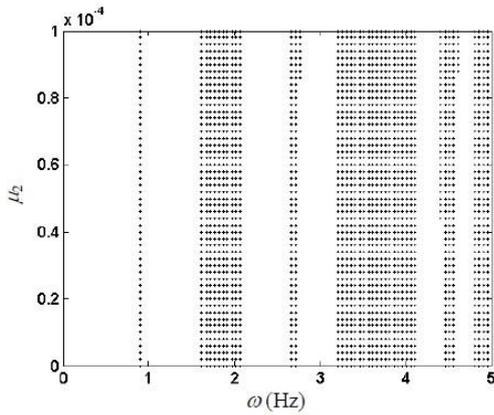
Fig. 9 Unstable region on the plane  $(\omega, \mu_2)$  of the controlled cable with multiple modes under random and periodic disturbances ( $\mu_1=1.5 \times 10^{-3}$ ,  $\zeta_{eq}=0.01$ )
