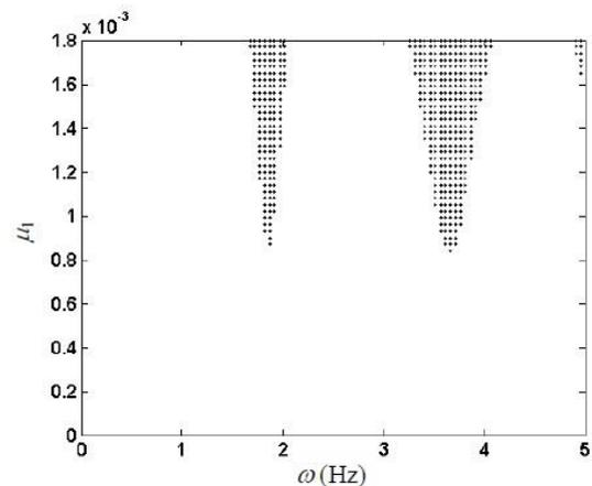
Fig. 7 Unstable region on the plane  $(\omega, \mu_1)$  of the controlled cable with multiple modes under random and periodic disturbances ( $\mu_2=0.05 \times 10^{-3}$ ,  $\zeta_{eq}=0.05$ )
