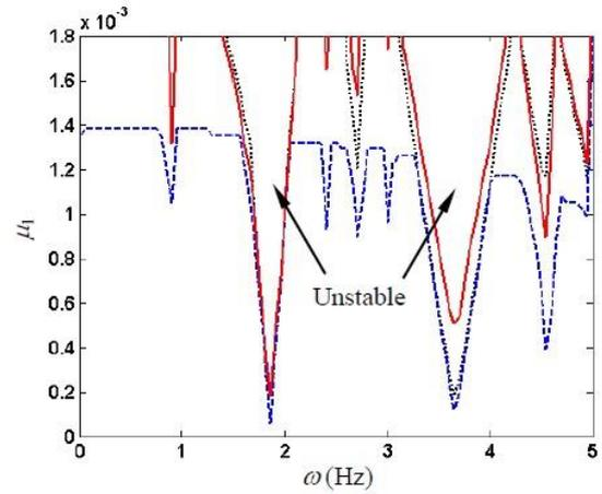
Fig. 17 Unstable region on the plane  $(\omega, \mu_1)$  of the controlled cable with various control damping and stiffness ( $\mu_2=0.05 \times 10^{-3}$ ) (solid line:  $\zeta_{eq}=0.01$ ,  $k_{eq}=0.1k_1$ ; dashed line:  $\zeta=0.002$ ,  $k_{eq}=0.1k_1$ ; dotted line:  $\zeta_{eq}=0.01$ ,  $k_{eq}=0$ )
