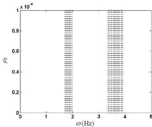
Fig. 10 Unstable region on the plane  $(\omega, \mu_2)$  of the controlled cable with multiple modes under random and periodic disturbances ( $\mu_1=1.5 \times 10^{-3}$ ,  $\zeta_{eq}=0.05$ )
