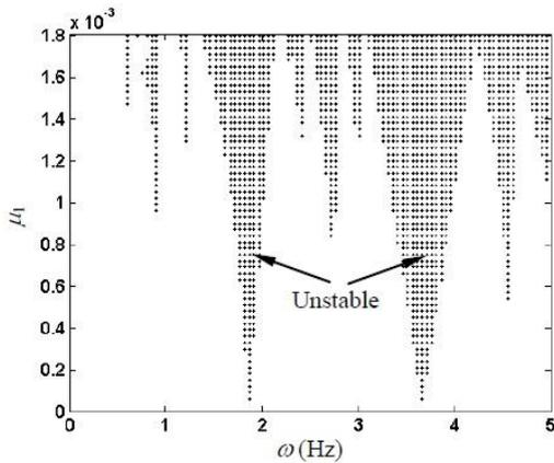
Fig. 3 Unstable region on the plane  $(\omega, \mu_1)$  of the uncontrolled cable with multiple modes under random and periodic disturbances ( $\mu_2=0.05 \times 10^{-3}$ )
