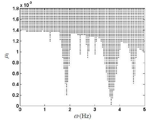
Fig. 12 Unstable region on the plane  $(\omega, \mu_1)$  of the controlled cable with multiple modes under random and periodic disturbances ( $\mu_2=0.05 \times 10^{-3}$ ,  $k_{eq}=0.2k_1$ )
