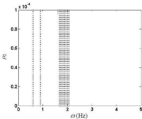
Fig. 4 Unstable region on the plane  $(\omega, \mu_2)$  of the uncontrolled cable with single mode under random and periodic disturbances ( $\mu_1=1.5 \times 10^{-3}$ )
