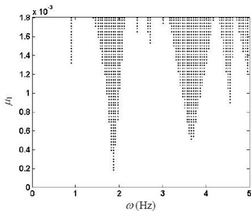
Fig. 16 Unstable region on the plane  $(\omega, \mu_1)$  of the controlled cable with multiple modes under random and periodic disturbances ( $\mu_2=0.05 \times 10^{-3}$ ,  $\zeta_{eq}=0.01$ ,  $k_{eq}=0.1k_1$ )
