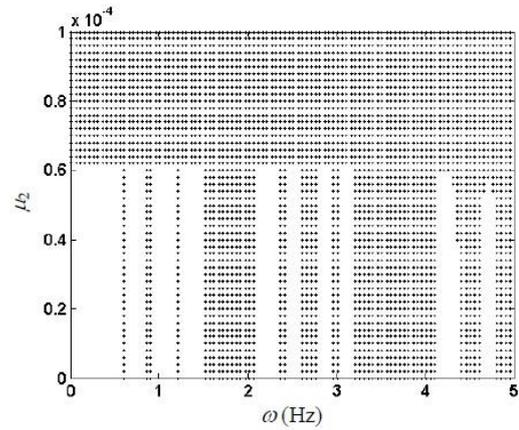
Fig. 5 Unstable region on the plane  $(\omega, \mu_2)$  of the uncontrolled cable with multiple modes under random and periodic disturbances ( $\mu_1=1.5 \times 10^{-3}$ )
