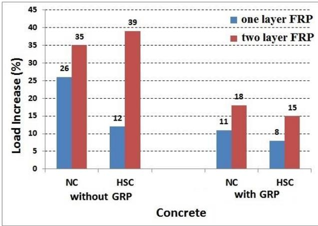
Fig. 8 FRP effect on compressive capacity of columns
