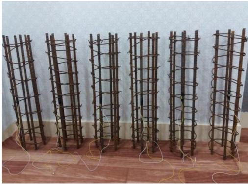
Fig. 2 Strain-gage installation on bars
