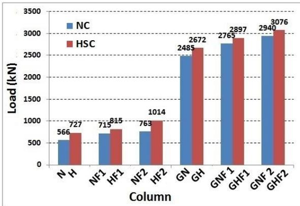
Fig. 9 Compressive capacity of columns
