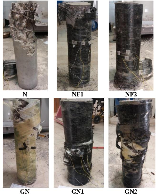
Fig. 14 Rupture of NC group of columns after loading
