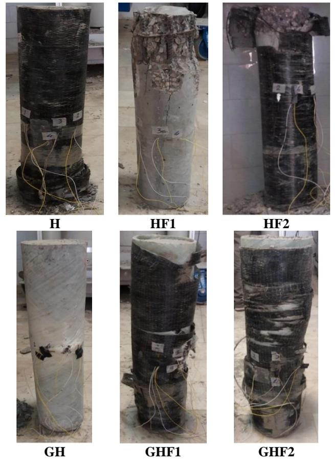
Fig. 15 Rupture of HSC group of columns after loading
