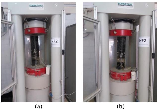
Fig. 7 Test setup and columns placement in jacks column NF2, (B) column HF2
