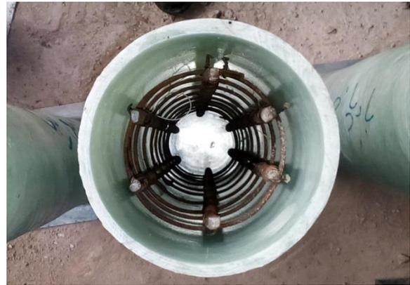
Fig. 4 Placement reinforcement inside CFRP casings and PVC framework
