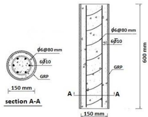
Fig. 1 Longitudinal and transverse sections of the research columns
