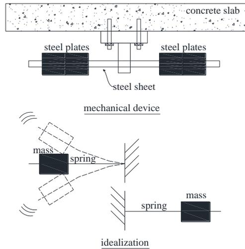
(b) Schematics of the mechanical system
