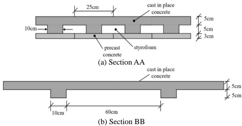
Fig. 2 Transversal sections of the concrete slab (see Fig. 1)
