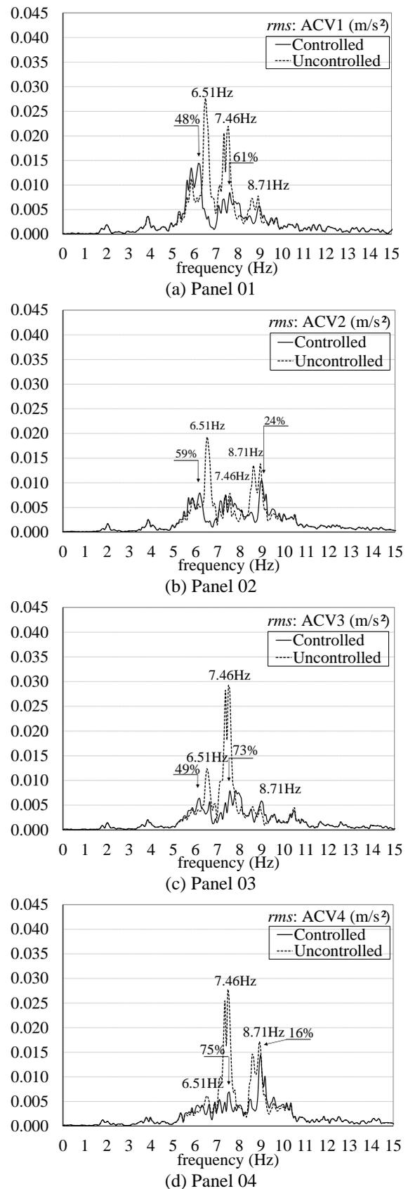
Fig. 12 Theoretical frequency responses of the four main slab panels of the uncontrolled and controlled structure subjected to human walking loading
