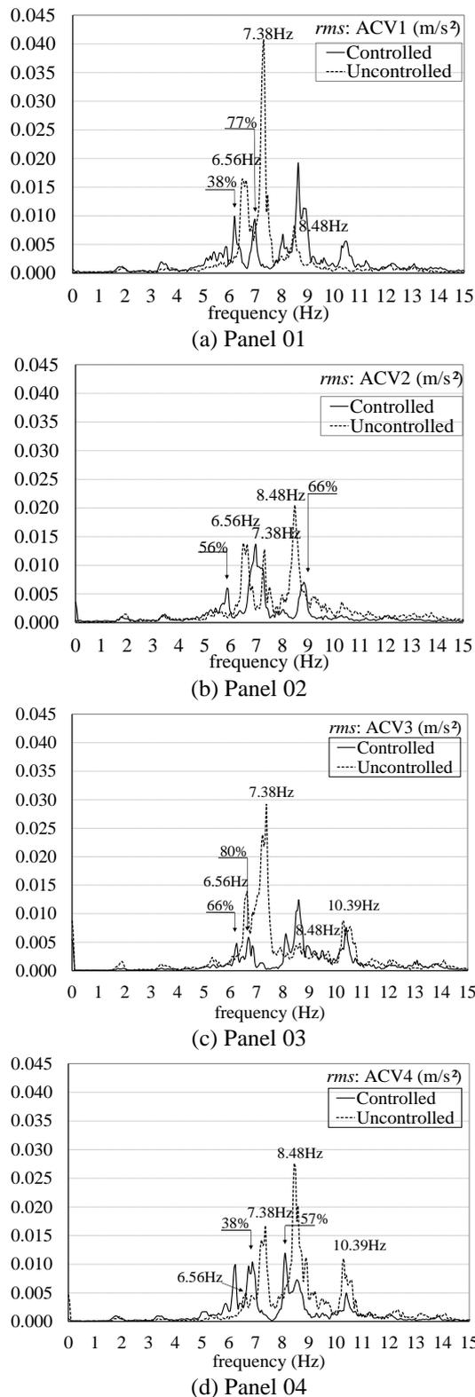
Fig. 10 Comparison of controlled and uncontrolled acceleration amplitudes at the center of the four main slab panels
