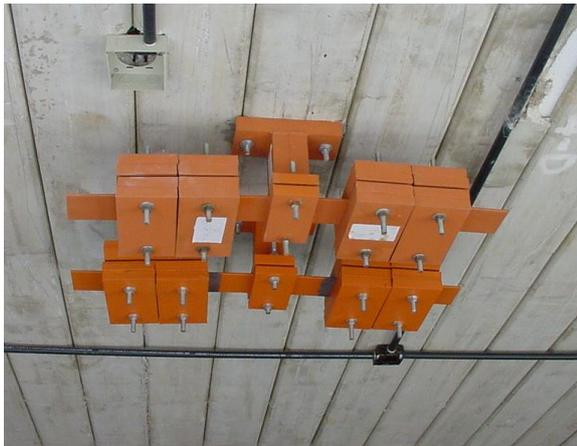
(a) Four SDAs installed at the bottom of one slab panel
