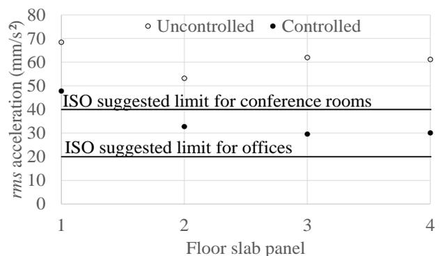
Fig. 11 Measured *rms* values of the vertical accelerations at the center of the slab panels in comparison with ISO 2631-2 (1989) recommendations
