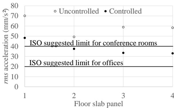
Fig. 13 Theoretical *rms* values of the vertical accelerations at the center of the slab panels in comparison with ISO 2631-2 (1989) recommendations
