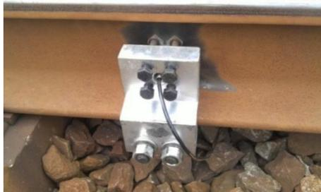
Fig. 13 The wheel-force monitoring sensor
