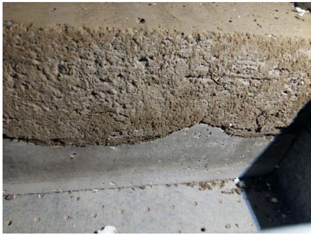
Fig. 12 Number of concrete tooth is 1 and its angularity is 15^\circ under normal stress of 150 KPa
