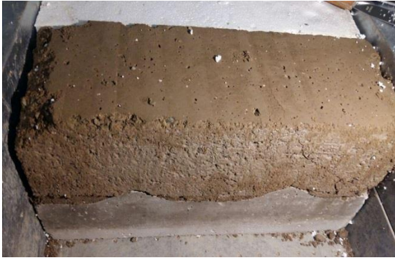
Fig. 17 Number of concrete tooth is 2 and its angularity is 30^\circ under normal stress of 300 KPa
