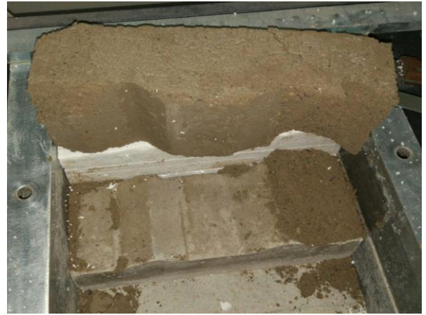
Fig. 15 Number of concrete tooth is 2 and its angularity is 15^\circ under normal stress of 300 KPa
