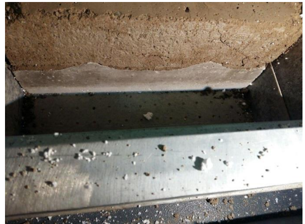
Fig. 16 Number of concrete tooth is 2 and its angularity is 15^\circ under normal stress of 150 KPa
