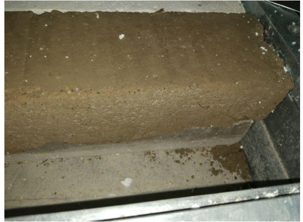
Fig. 14 Number of concrete tooth is 2 and its angularity is 15^\circ under normal stress of 150 KPa
