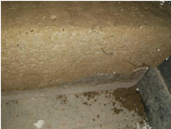
Fig. 18 Number of concrete tooth is 2 and its angularity is 30^\circ under normal stress of 500 KPa
