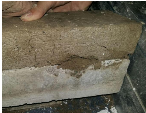
Fig. 10 Number of soil tooth is 1 and its angularity is 30^\circ under normal stress of 80 KPa
