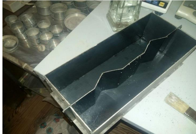
Fig. 2 The mold used for sample preparation
