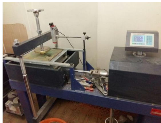
Fig. 7 Direct shear test apparatus
