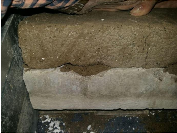
Fig. 11 Number of soil tooth is 2 and its angularity is 30^\circ under normal stress of 80 KPa
