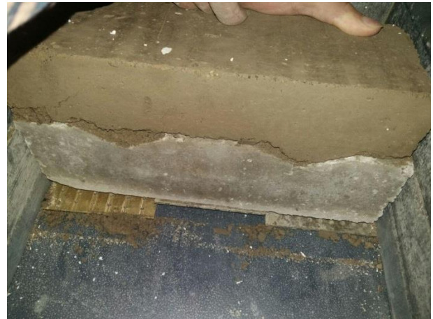
Fig. 9 Number of soil tooth is 2 and its angularity is 15^\circ under normal stress of 80 KPa
