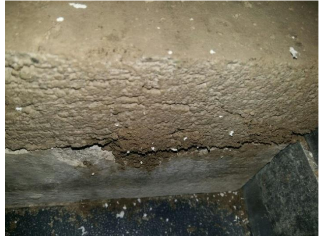
Fig. 8 Number of soil tooth is 1 and its angularity is 15^\circ under normal stress of 80 KPa
