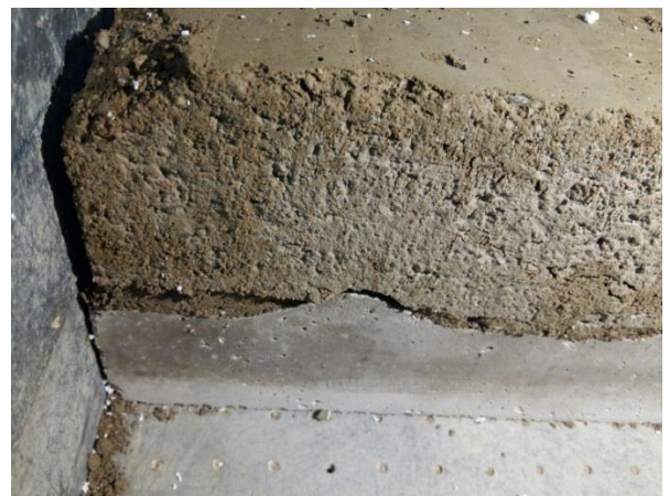
Fig. 13 Number of concrete tooth is 1 and its angularity is 15^\circ under normal stress of 300 KPa
