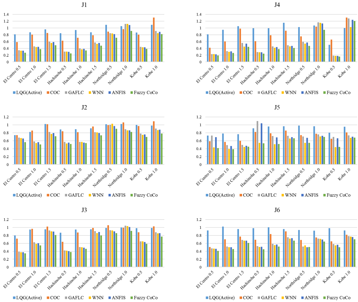
Fig. 13 Comparison of performance criteria J_1 – J_6 of Fuzzy Cooperative Coevolution (Fuzzy CoCo), Adaptive Neuro-Fuzzy Inference System (ANFIS), Wavelet Neural Network (WNN), fuzzy logic controller optimized by genetic algorithm (GAFLC), Clipped Optimal Control (COC) and Linear Quadratic Gaussian (LQG) methods
