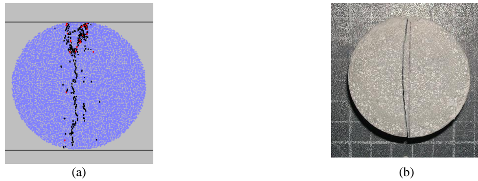
Fig. 2 The failure pattern in the (a) numerical model and (b) experimental samples
