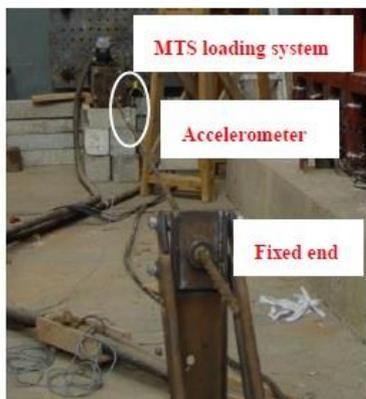
Fig. 6 The cable test setup
