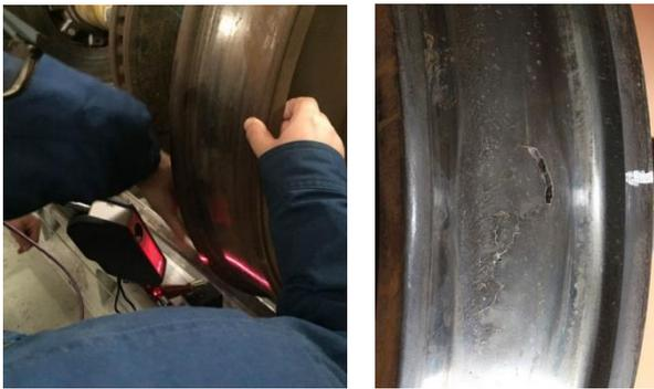
Fig. 9 Offline wheel tread inspection: left panel - radius deviation measurement; right panel - local defect detected
