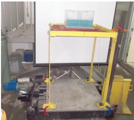
Fig. 7 The test setup for forced vibration tests on TLD-structure systems
