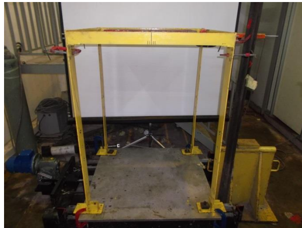
Fig. 6 The bare steel structure which is installed on the platform of a shake table
