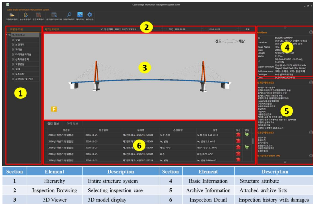
Fig. 11 BIM-based maintenance information management system design and realization — Software interface
