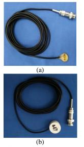
Fig. 2 Photos of a PZT patch and a smart aggregate: (a) A PZT patch with a BNC connector and (b) AnSA with a BNC connector
