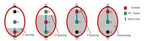
Fig. 3 Detection schematic of active sensing based grouting compactness monitoring
