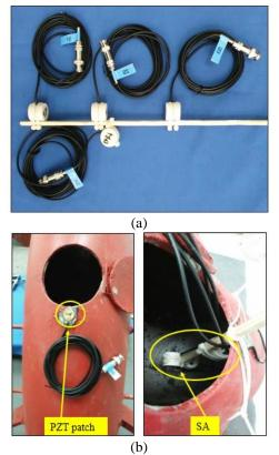
Fig. 4 Transducer installation: (a) SAs supported with a wood stick and (b) A photo of mounted PZT patch and installed SAs
