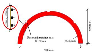
Fig. 5 Dimensions of the steel tube specimen and the location of the transducers
