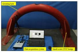
Fig. 6 Experimental setup
