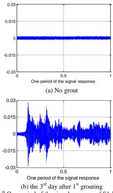
Fig. 7 One period of the signal response of S1-P1
