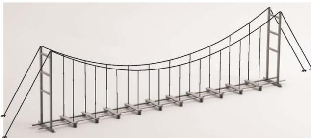
Fig. 1 CAD view of the studied suspension bridge
