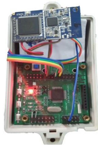
Fig. 8 Hardware design of wireless sensing unit
