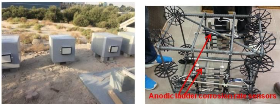
Fig. 3 Anodic ladder corrosion sensors installed in concrete blocks for atmospheric zone at KISR field research station
