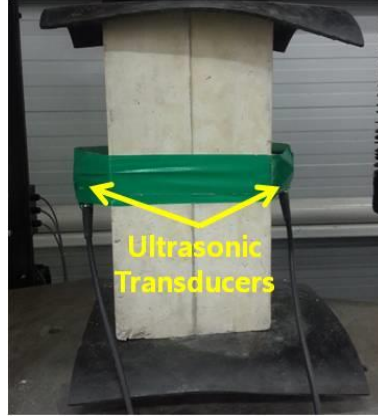
Fig. 2 Uni-axial Compression Test Setup
