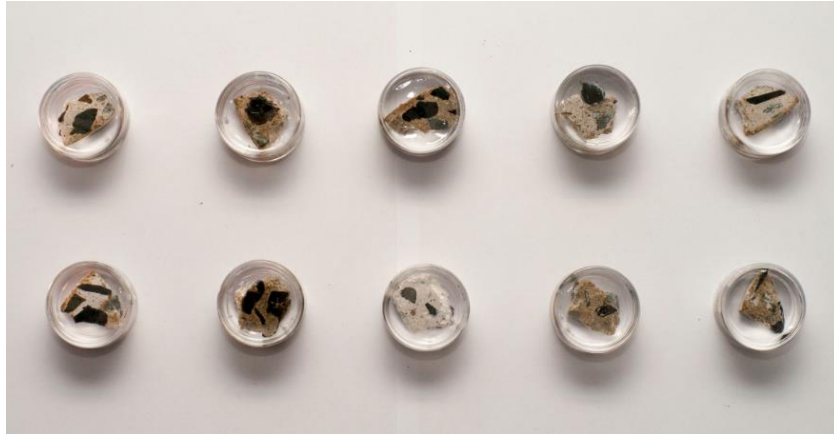
Fig. 5 Polymer molds incorporating concrete samples for SEM analysis
