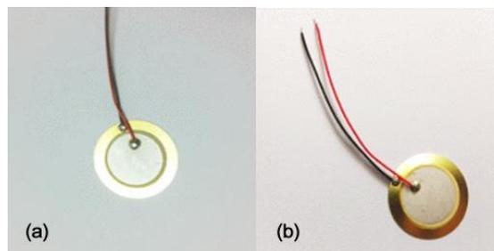
Fig. 1 PZT sensor (a) before coating and (b) after coating with acrylic resin
