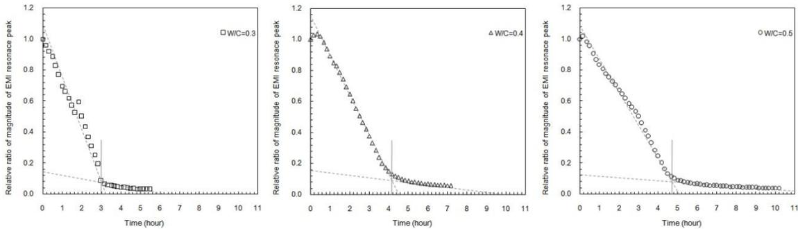
Fig. 7 Magnitude of EMI resonance peak as function of material age
