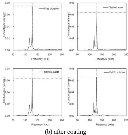
Fig. 2 EMI signatures of PZT sensor under various conditions
