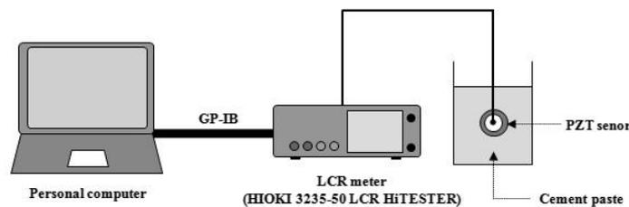
Fig. 3 Test setup for measuring EMI of PZT sensor
