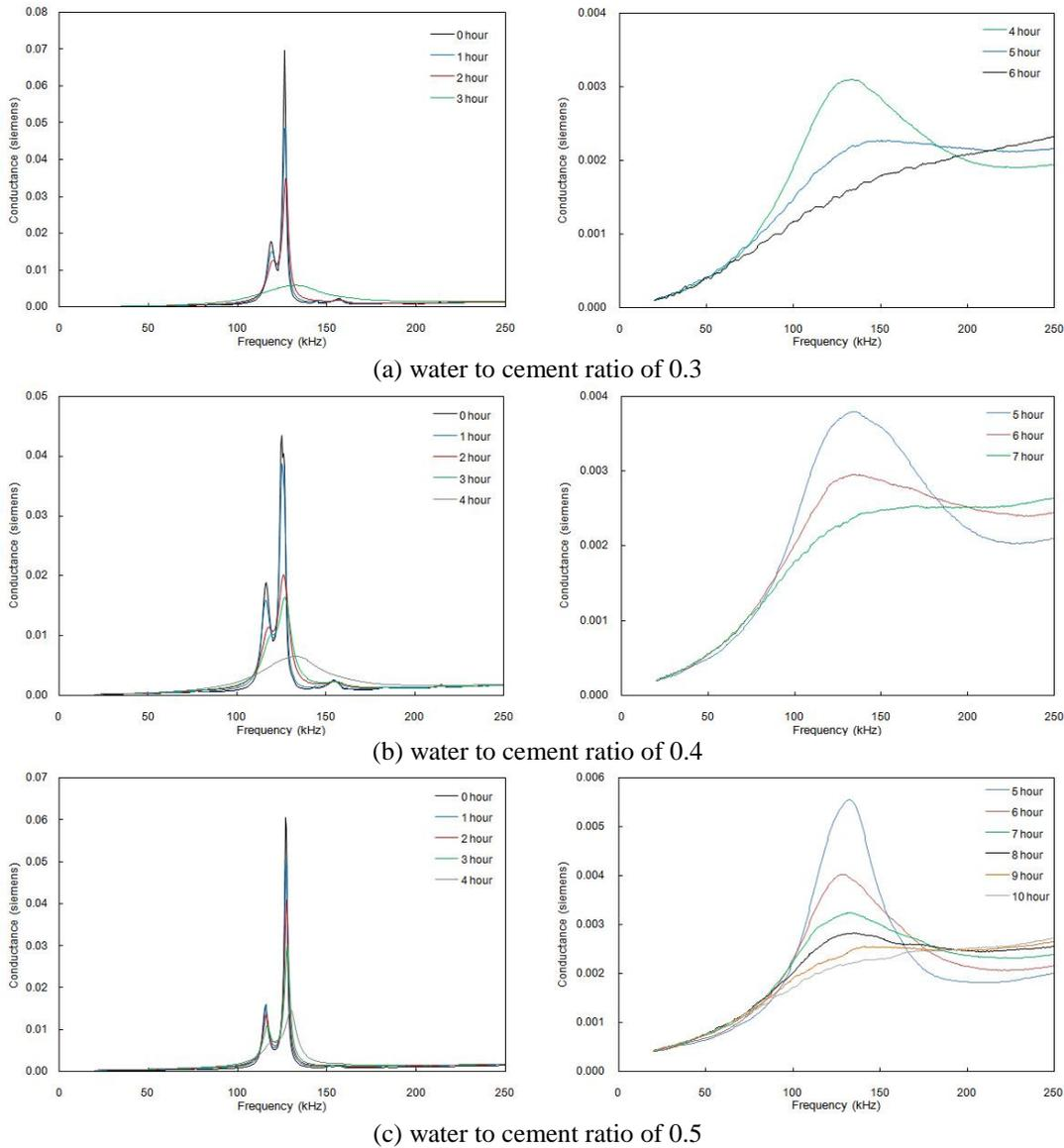
Fig. 6 EMI signatures of PZT sensor embedded in cement pastes
