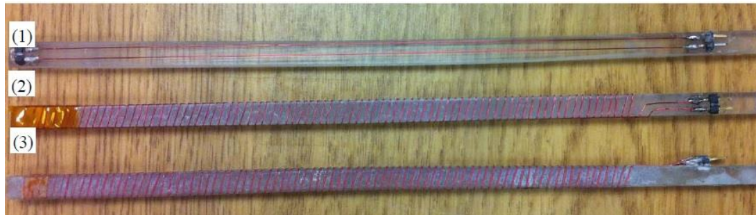
Fig. 9 Photo of spiral-shaped TDR probe
