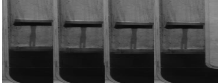
Fig. 6 The consecutive images for the variation of free surface of MR-fluid under test
