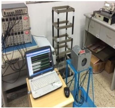
Fig. 7(a) Lab experiment of a 5-story building
