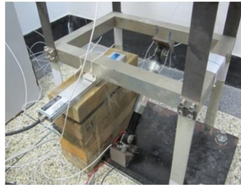
Fig.7(b) MR damper installed in the 1st story
