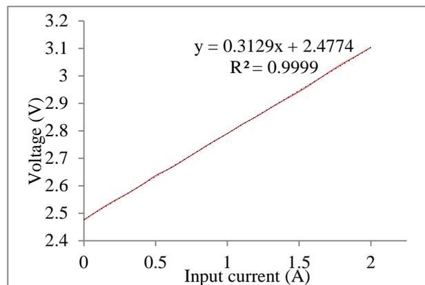
Fig. 6 Calibration curve of current sensor
