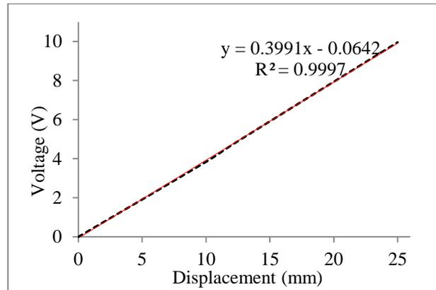
Fig. 5 Calibration curve of displacement sensor
