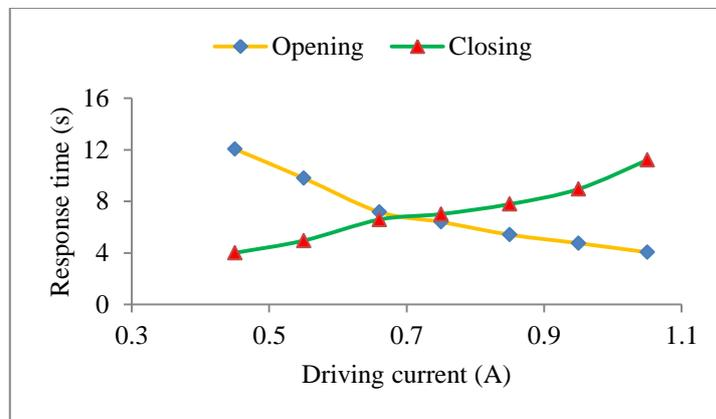
Fig. 13 Response time of the gripper for open and close operations
