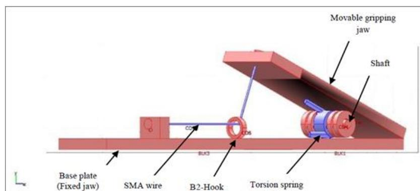
Fig. 1 CAD model of the SMA actuated gripper with torsion spring
