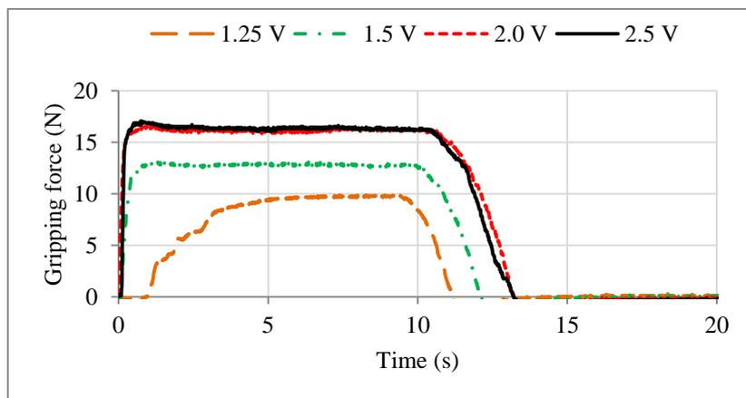
Fig. 11 Force response of SMA actuated gripper at different voltages
