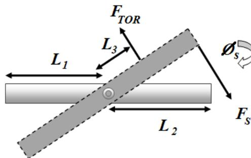
Fig. 2 Free body diagram of rotary upper gripping jaw under steady state
