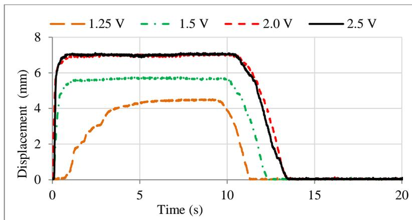
Fig. 9 Response of gripper at different voltage levels
