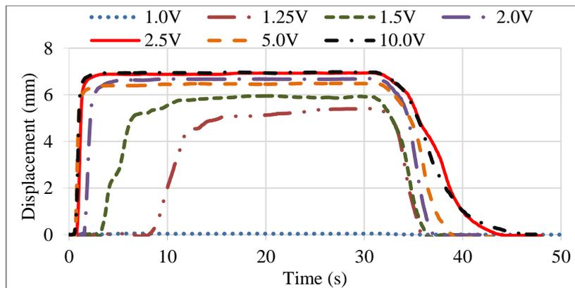
Fig. 7 Response of the gripper at different voltage levels
