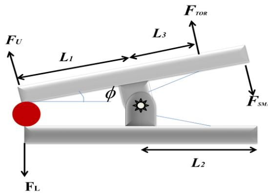
Fig. 3 Free body diagram of SMA gripper holding object
