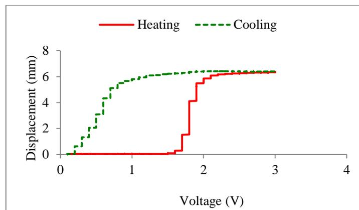
Fig. 14 Response of the gripper for one complete cycle
