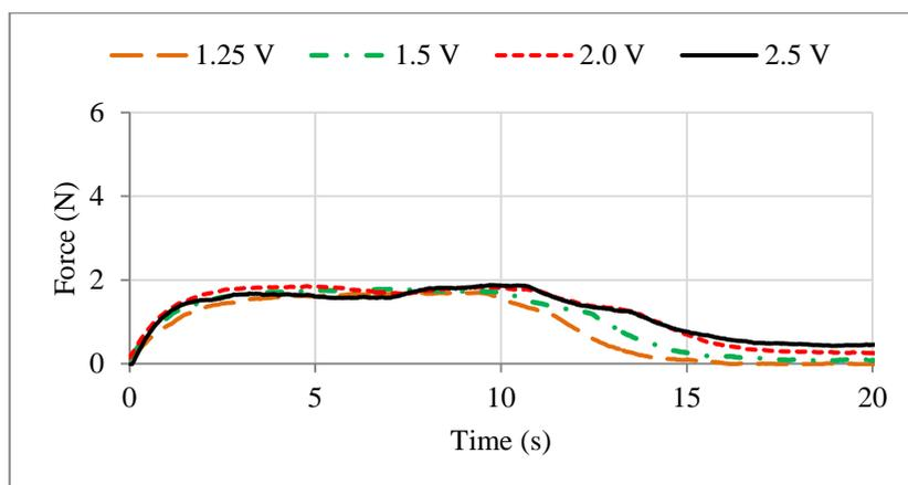
Fig. 10 Force response of SMA wire at different voltage levels
