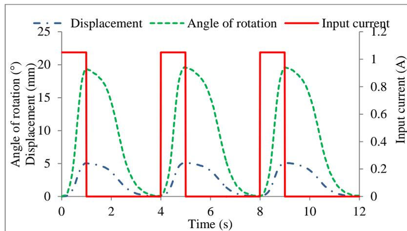
Fig. 17 Separation of the movable jaw of the gripper when the SMA wire is actuated under controlled forced air
