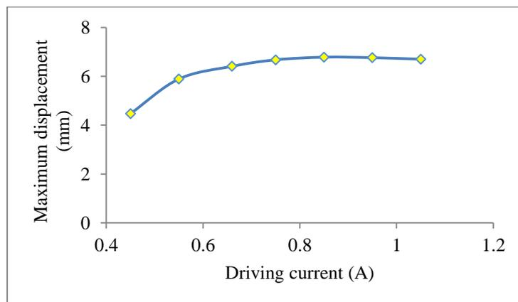
Fig. 12 Response of the gripper for increasing driving current
