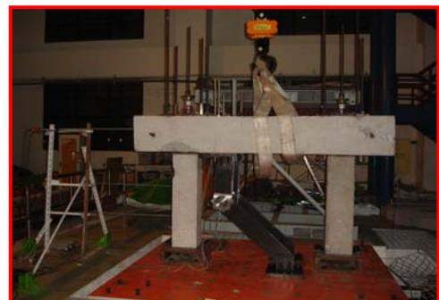
Fig. 2 Lateral resistance of a self-centering designed bridge
