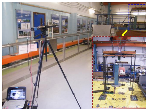
Fig. 10 Experimental setup of shaking table tests
