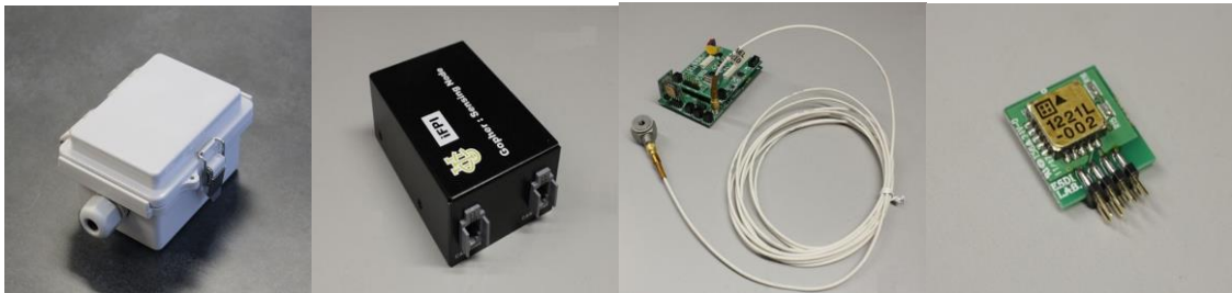
(a) for Outdoor, (b) for Indoor, (c) PCB w/PZT and (d) Pluggable sensor
