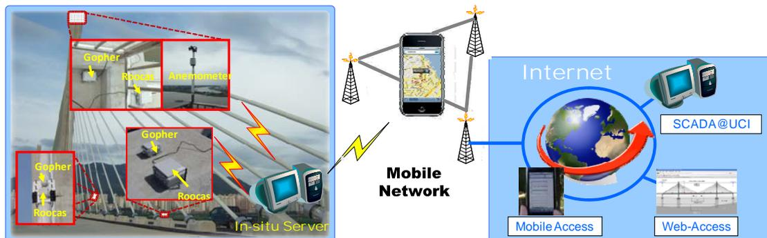
Fig. 13 Remote Monitoring Topology: Smartphone or Web access through internet
