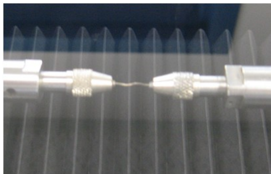
Fig. 12 Torsion induced buckling for the ‘fixed’ end condition (Chapman 2011)
