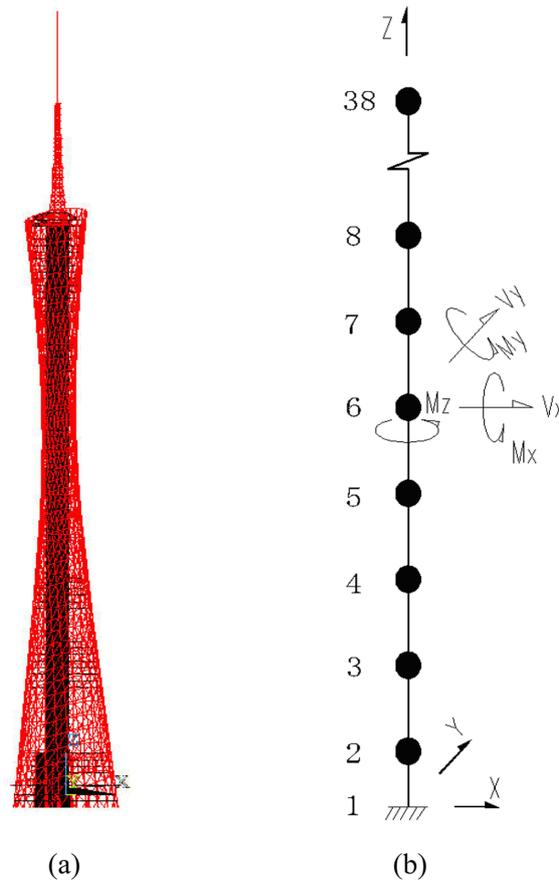
Fig. 2 The FE model of the Canton Tower: (a) Full-order 3D FE Model and (b) reduce-order FE Model
