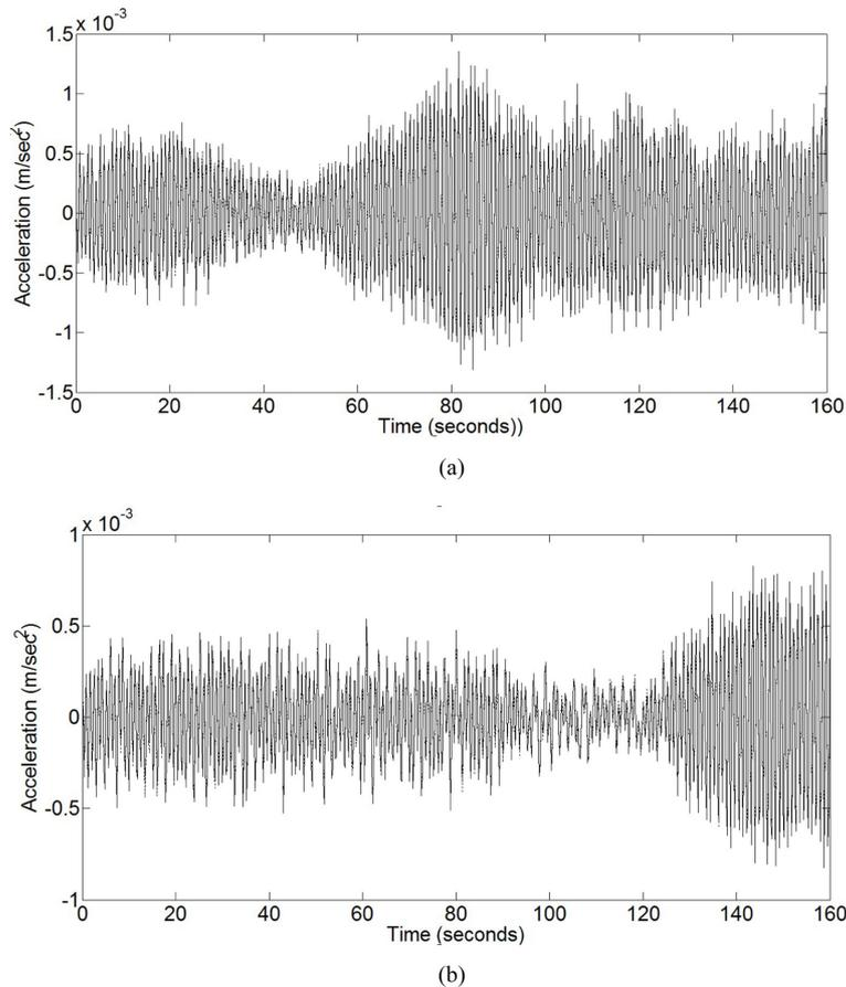
Fig. 4 Comparisons of acceleration responses at desired location: (a) Comparison of acceleration responses at Sensor No. 9 and (b) comparison of acceleration responses at Sensor No. 12
