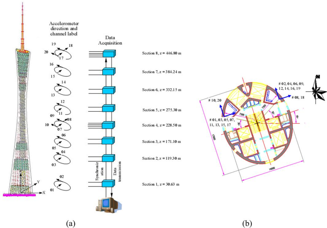
Fig. 3 Deployment of accelerometers on the Canton tower: (a) Position of accelerometers and (b) direction of measured accelerations and channel labels
