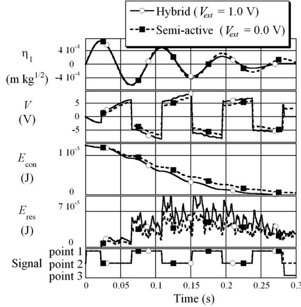
Fig. 5 Efficiency comparison of single-mode vibration suppression
