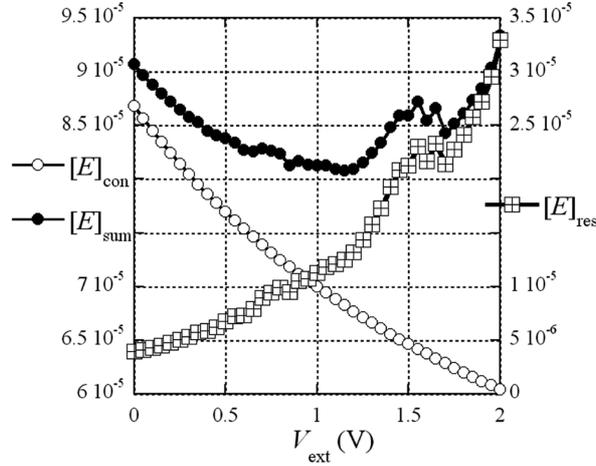
Fig. 6 Energy evaluation as a function of external voltage (controlled-mode energy  $[E]_{con}$ , residual-mode energy  $[E]_{res}$ , and sum of all energies  $[E]_{sum}$ )
