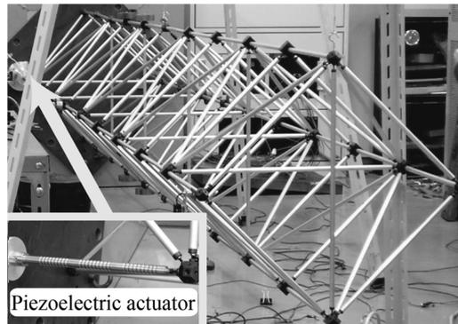
Fig. 3 Experimental setup for hybrid vibration suppression and magnified view of piezoelectric actuator
