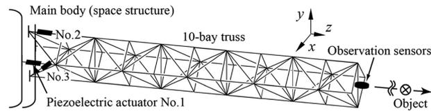
Fig. 1 Example of MDOF systems (extension mast stretching from a main body, e.g., astronomical satellite and space station): 10-bay truss with multiple actuators at fixed end, and sensors observing far-away astronomical objects
