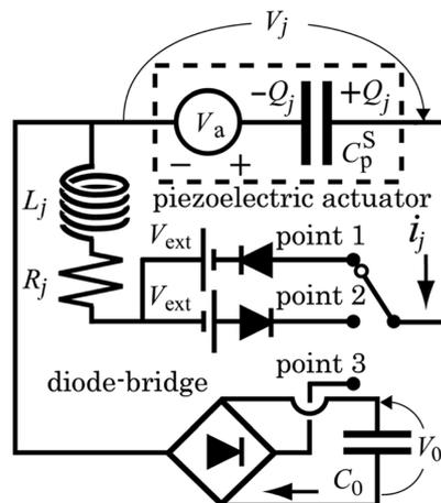
Fig. 2 Energy-storing electric circuit for hybrid vibration suppression
