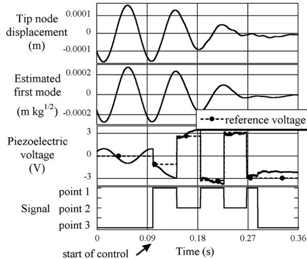
Fig. 8 Suppression experiment of original hybrid method (without displace-offset prevention) that is cited from (Makihara 2005)
