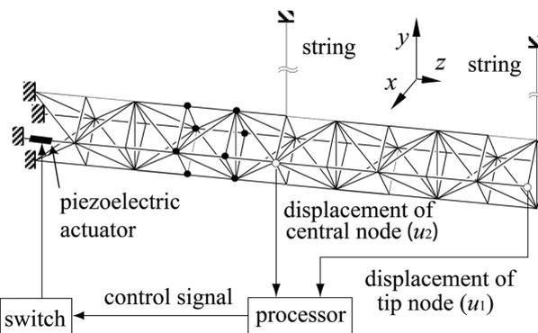
Fig. 4 Control flow of hybrid vibration suppression experiment
