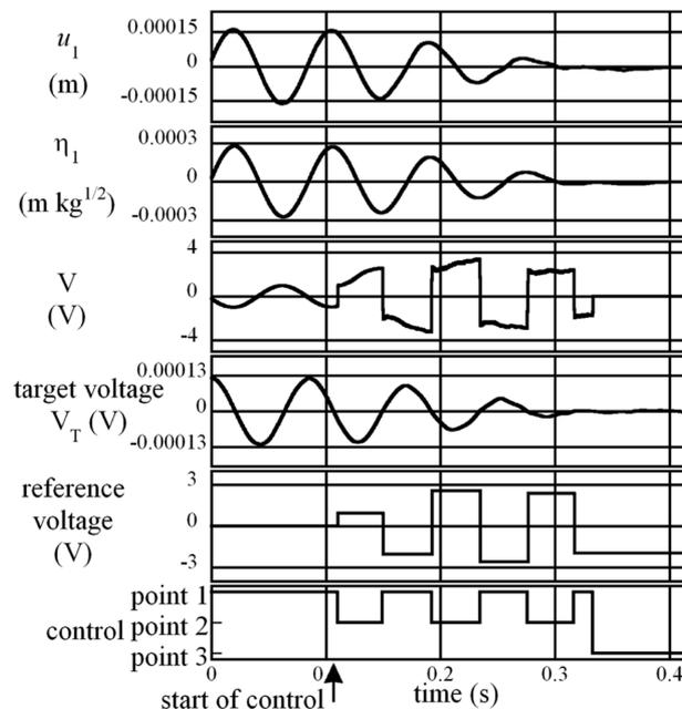
Fig. 7 Suppression experiment of new hybrid method using energy-storing circuit (with displace-offset prevention)
