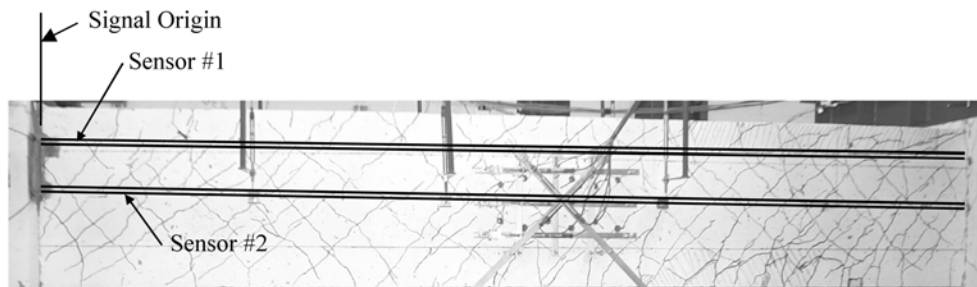
Fig. 10 SE test region after Load Cycle 4C
