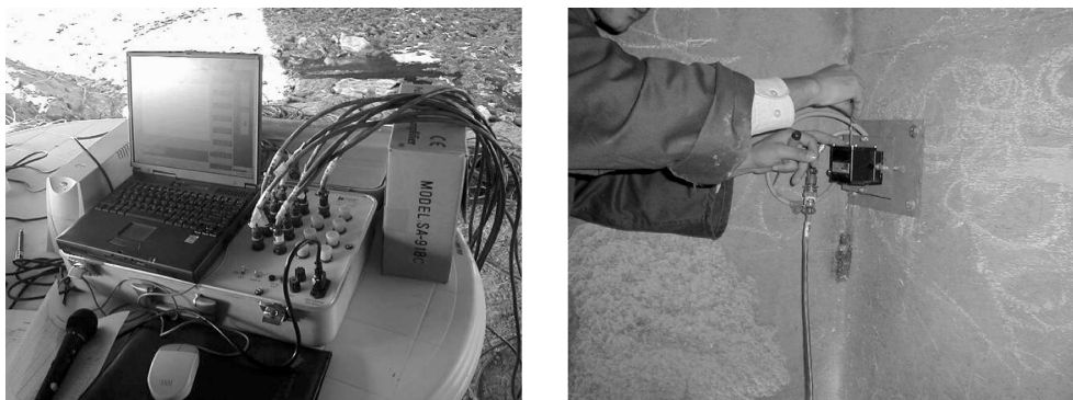
Fig. 7 Data acquisition system and an example of accelerometer attached to the bridge
