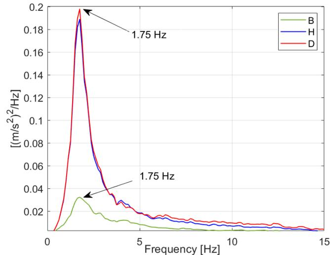
Fig. 5 PSD functions computed from sensor B (on pitch axis), D (on roll axis) and H (above wheel). Pitch and bounce peaks are highlighted
