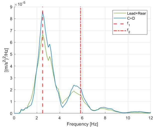
Fig. 8 Comparison of the PSD functions computed from two different signals: the green line refers to a signal obtained averaging the raw data from the sensors placed on the lead (C, E, F) and on the rear (D, G, H); the blue line refers to a signal obtained averaging the raw data from sensors C and D. The dashed lines highlight the first two bending frequencies of the bridge. Refer to Fig. 3 for the positioning of the sensors
