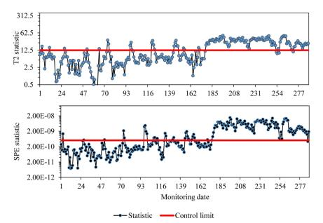
Fig. 14 Control charts of hybrid modeling (PCA-KPCA) obtained using LSSEs features for Yonghe bridge at Sensor-2
