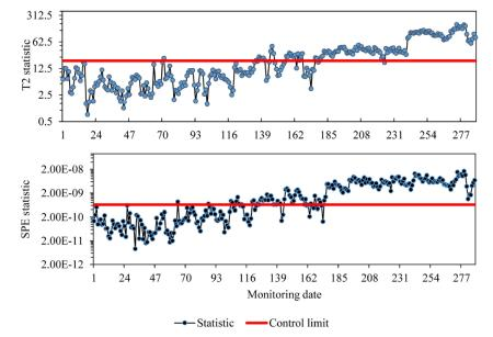
Fig. 13 Control charts of hybrid modeling (PCA-KPCA) obtained using SSCs features for Yonghe bridge at Sensor-2
