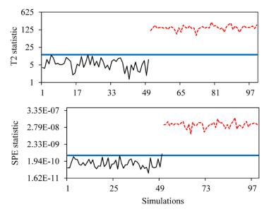
Control limit — Undamaged ----- Damaged
