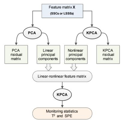
Fig. 1 Schematic for hybrid modeling based on PCA and KPCA
