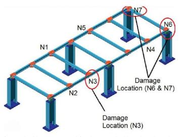
Fig. 3 Node numbers for steel grid structure used for the numerical benchmark study (Gul and Catbas 2011)
