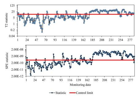
Fig. 15 Control charts of hybrid modeling (PCA-KPCA) obtained using LSSEs features for Yonghe bridge at Sensor-4
