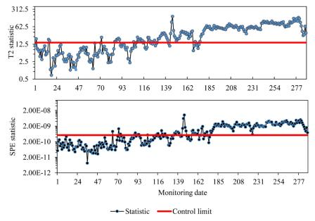
Fig. 12 Control charts of hybrid modeling (PCA-KPCA) obtained using SSCs features for Yonghe bridge at Sensor-1
