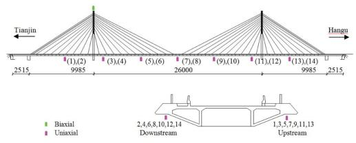
Fig. 11 Elevation of Tianjin Yonghe Bridge with the main dimensions and accelerations health monitoring system (Kaloop and Hu 2015)
