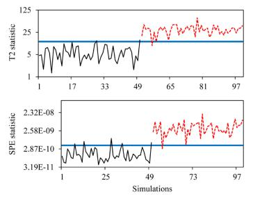
Control limit — Undamaged ------ Damaged
