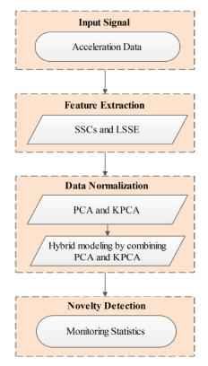
Fig. 2 Flowchart showing the methodology for damage identification
