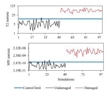
Fig. 7 Control charts of hybrid modeling (PCA-KPCA) obtained using LSSEs features for Case A at node N1
