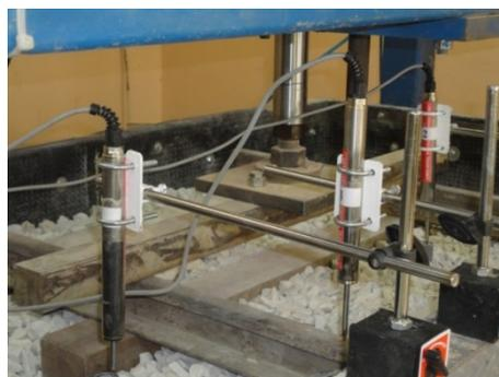
Fig. 5 Load spreader beam and Linear Variable Differential Transformers (LVDTs)
