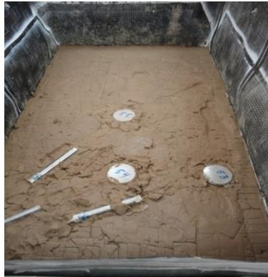
Fig. 7 Earth pressure cells
