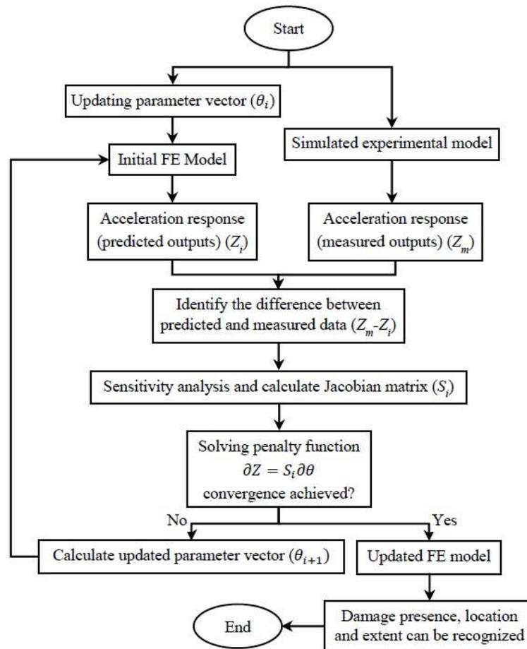
Fig. 1 Flowchart for the model updating procedure
