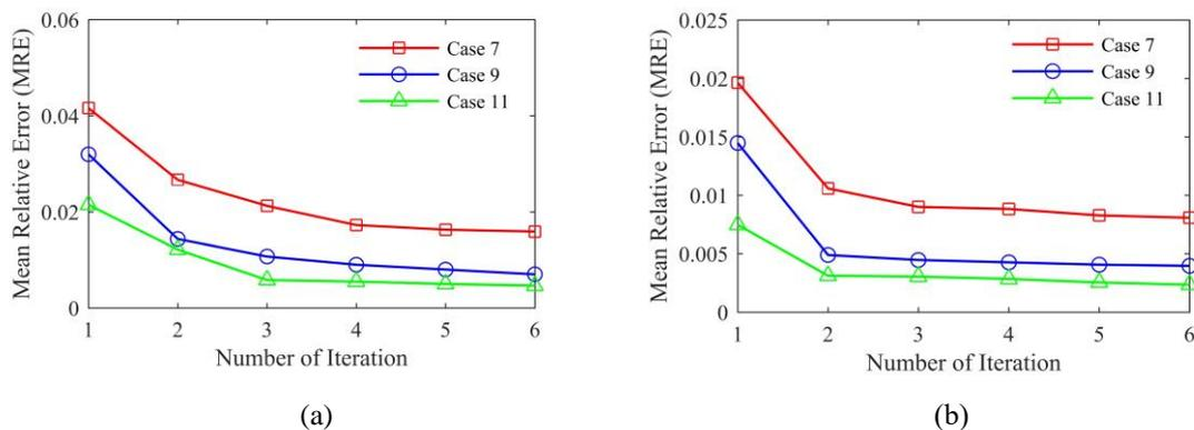
Fig. 7 Convergence graphs of FE model updating process: (a) Flat double layer grid, (b) Double layer diamatic dome
